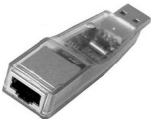
8-Rasm. 100Base-TX standartli USB-portiga ulanuvchi tarmoq adapteri.
