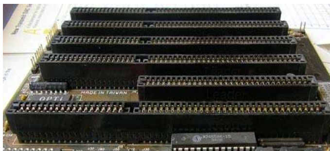
3-rasm. ISA shina: 4 ta 16 bitli va 1 ta 8 bitli razyom
