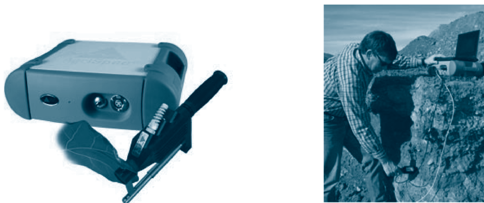
Figure 8.10 The AgriSpec® portable NIR spectrometer with plant probe and leaf clip assembly (left) and in use in a soilpit (right) (Photos courtesy of Analytical Spectral Devices, Inc., Boulder, Colorado, USA. Copyright © Analytical Spectral Devices, Inc. All rights reserved.).
