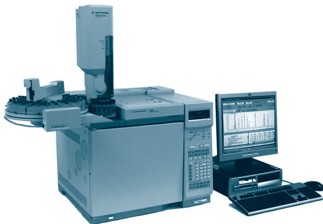
Figure 3.8 Agilent 6890 gas chromatograph (© Copyright 2006 Agilent Technologies, Inc. Reproduced with permission).
