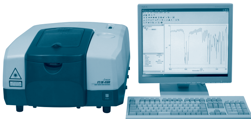
Figure 2.16 An FTIR spectrometer (Reproduced by kind permission of Jasco Corporation).
