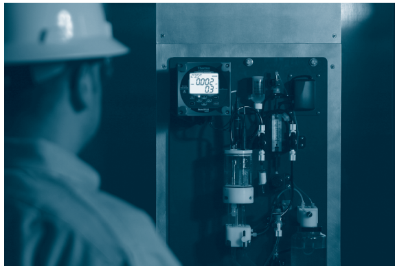
Figure 9.6 On-line low-level measurements of sodium using the Orion ionplus 2111LL on-line ion-selective sodium electrode (Reproduced by kind permission of Thermo Electron Corp).
