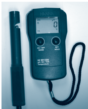
Figure 8.9 The portable HI-991300 conductivity meter (Reproduced with permission of Sheen Instruments Ltd).
