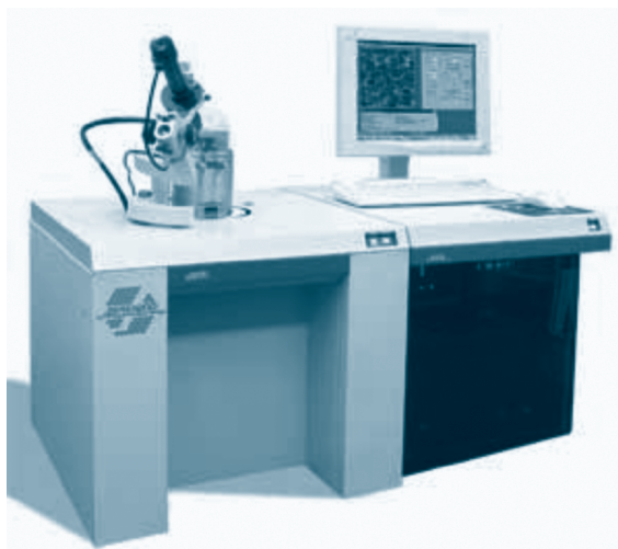
Figure 4.10 The JSPM-5200 scanning probe microscope can be configured as either an atomic force microscope (AFM) or scanning tunnelling microscope (STM) by changing the tip (Image courtesy of Jeol).
