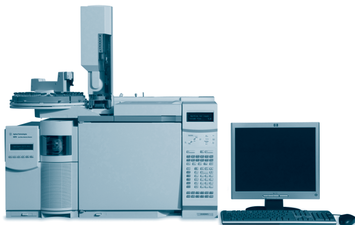
Figure 3.39 Agilent 5975 Inert MSD and Agilent 6890 GC with PC (© Copyright 2006, Agilent Technologies, Inc. Reproduced with permission).
