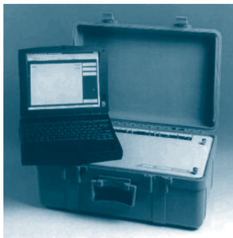
Figure 7.12 The MS-200 portable mass spectrometer (Reproduced by permission of Kore Technologies).
