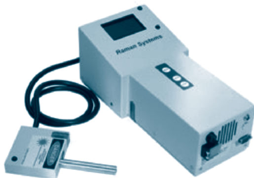
Figure 7.8 The RSL Plus portable Raman spectrometer (Reproduced by permission of Raman Systems).
