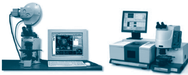
Figure 4.11 The SpectraView® spectral imaging instrument from Applied Spectral Imaging and the FTIR spectral imaging system from Varian (Reproduced by permission of Applied Spectral Imaging and Varian Inc.).
