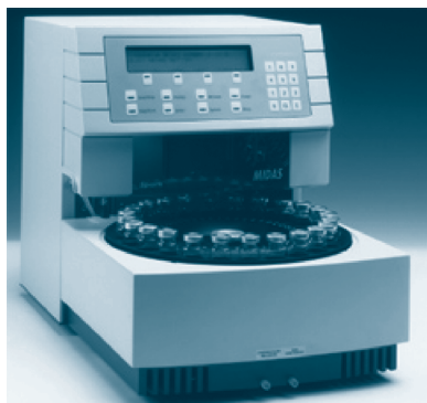
Figure 3.13 The Smartline 3900 autosampler module (Reproduced by permission of Flowspek/Knauer).
