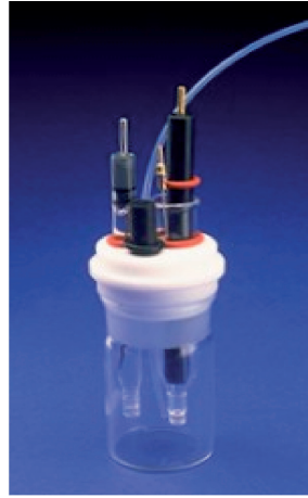
Figure 5.6 Schematic diagram and photograph of a three-electrode voltammetric cell (Figure used by kind permission of Dr. Marco Cardosi, Dept of Biological Sciences, University of Paisley, UK; photograph courtesy of BAS Inc., USA.).
