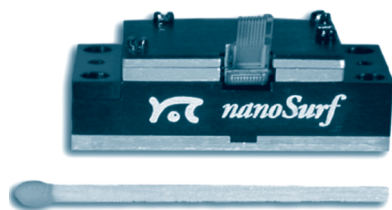
Figure 10.11 The AFM scanner from Nanosurf will be part of the miniaturised suite of microscopic instrumentation on the Phoenix space mission to Mars (Reproduced by permission of Nanosurf).
