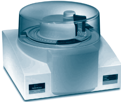
Figure 6.6 The Jade DSC (Reproduced by permission of Perkin Elmer Inc.).
