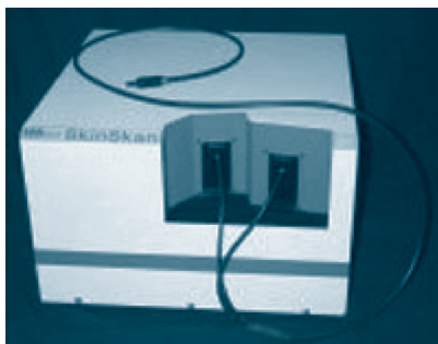
Figure 8.8 The portable SkinScan spectrofluorometer (Reproduced by permission of HORIBA Jobin Yvon).
