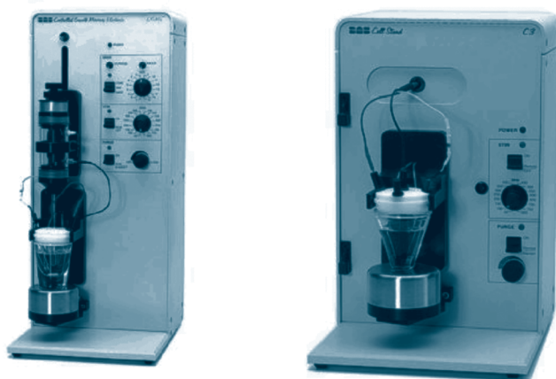
Figure 5.7 Controlled growth mercury electrode for polarography and C-3 cell stand for voltammetry (Reproduced by permission of BAS Inc.).
