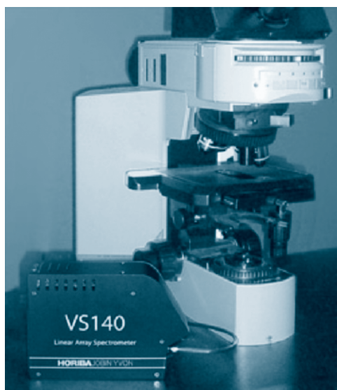
Figure 7.21 The VS140 interfaced to a microscope to give an imaging spectrometer (Reproduced by permission of HORIBA Jobin Yvon).
