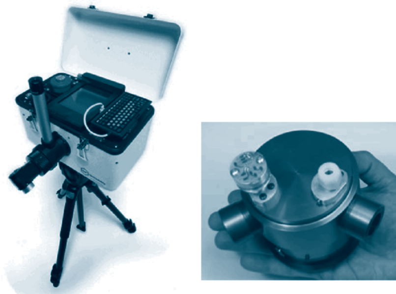
Figure 7.6 The Model 102 portable FTIR spectrometer and a close-up of the small interferometer used in the Model 102 (Photographs reproduced by permission of D&P Instruments).
