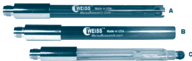
Figure 5.2 A variety of shapes and sizes of pH electrodes is available, e.g. epoxy body (A), flat (B) or round (C) bulb shaped pH electrodes (Reproduced by permission of Weiss Research).
