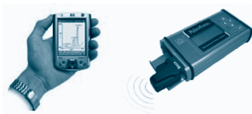
Figure 7.24 The wireless PalmSens potentiostat–galvanostat (right) and the pocket PC used to control it (left) (Reproduced by permission of Palm Instruments).
