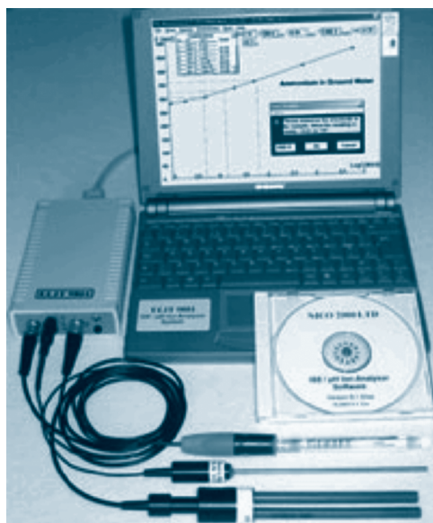
Figure 5.4 The ELIT ion/pH analyser system (Different ISEs can be attached as required. Reproduced by permission of Nico 2000 Ltd.).
