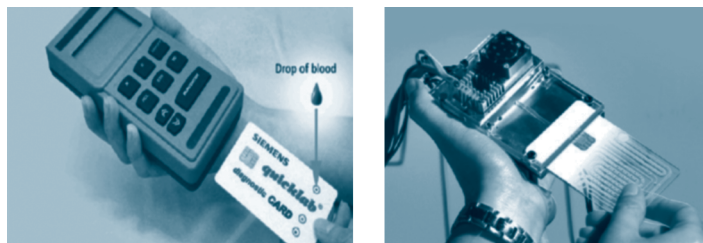
Figure 10.13 The Quicklab device and diagnostic card; on the right, both the device and card are uncovered revealing the inner components of the handheld reader and the microfluidics on the chip (Photographs: Courtesy of Siemens AG).
