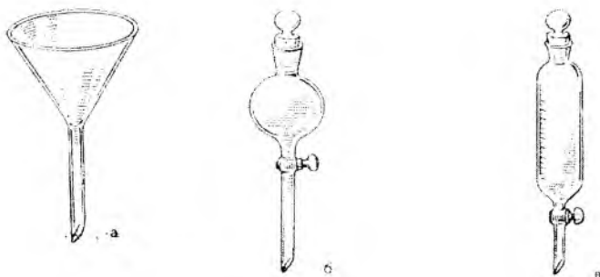
Rasm. 7. Voronkalar: a – kimyoviy; b — tomizgich; v - ajratkich.
