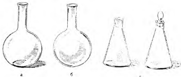
Rasm. 4. Kolbalar: a – tagi yassi; b – tagi dumaloq; v – konussimon.
