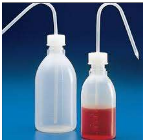
5-rasm Suv purkagichlar (yoki yuvgich)
