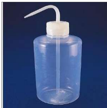
5-rasm Suv purkagichlar (yoki yuvgich)
