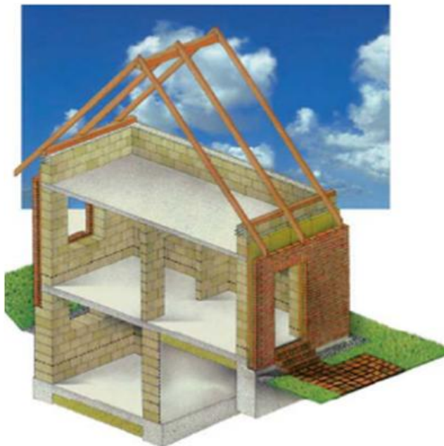
3-rasm. Yuk ko`taruvchi devorli bino
