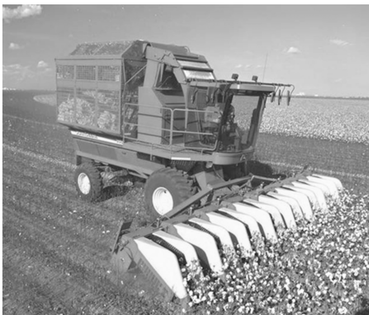
6.4 Typical stripper harvester for cotton.
