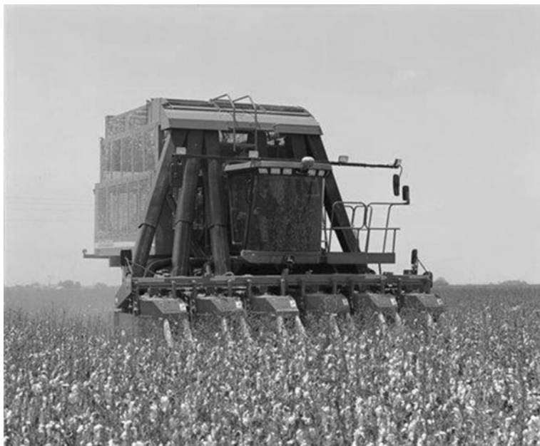
6.3 Typical spindle-type mechanical harvester for cotton.
