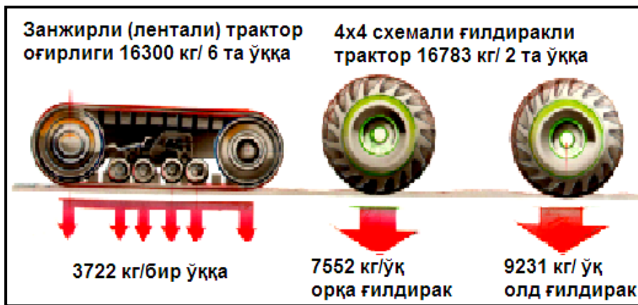
1.18-rasm. Traktor yurish qismining tuproqning chuqur zichlanishiga ta'siri
