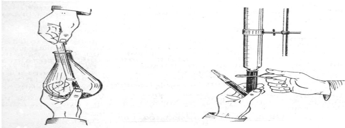
31-rasm. a) konussimon kolbaga tuproqni solish, b) eritmani titrlash uchun ishlatiladigan byuretka
