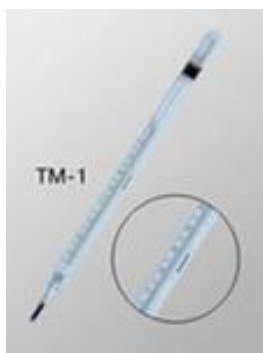
2-rasm. Maksimal termometr TM-1
