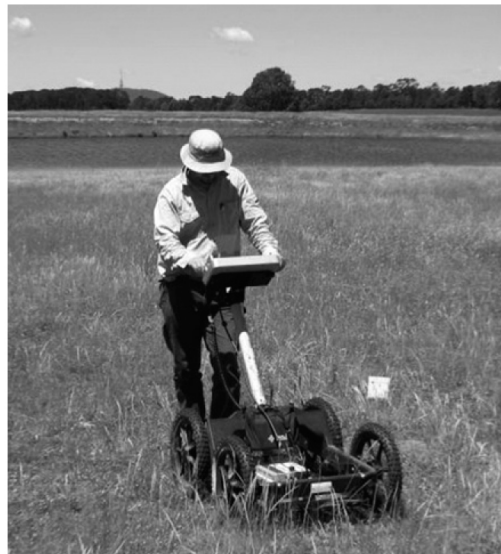
Fig. 11. A ground-penetrating radar (GPR) system [after Viscarra Rossel et al. , 2011].
