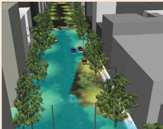
Figure 13.21 Virtual London law enforcement analysis: 3-D visualization of closed circuit television viewshed (green) and street illumination (Courtesy: Christian Castle, John Calkins, and ESRI)
