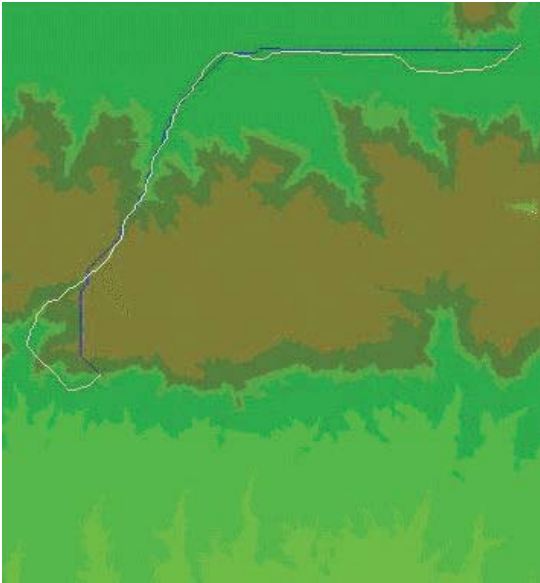
Figure 15.20 Solution of a least-cost path problem. The white line represents the optimum solution, or path of least total cost, across a friction surface represented as a raster, and using the queen's-case move set (eight possible moves). Brown denotes the highest friction. The blue line is the solution when cells are aggregated in blocks of 3 by 3, and the problem is solved on this coarser raster (Reproduced by permission of Ashton Shortridge)
