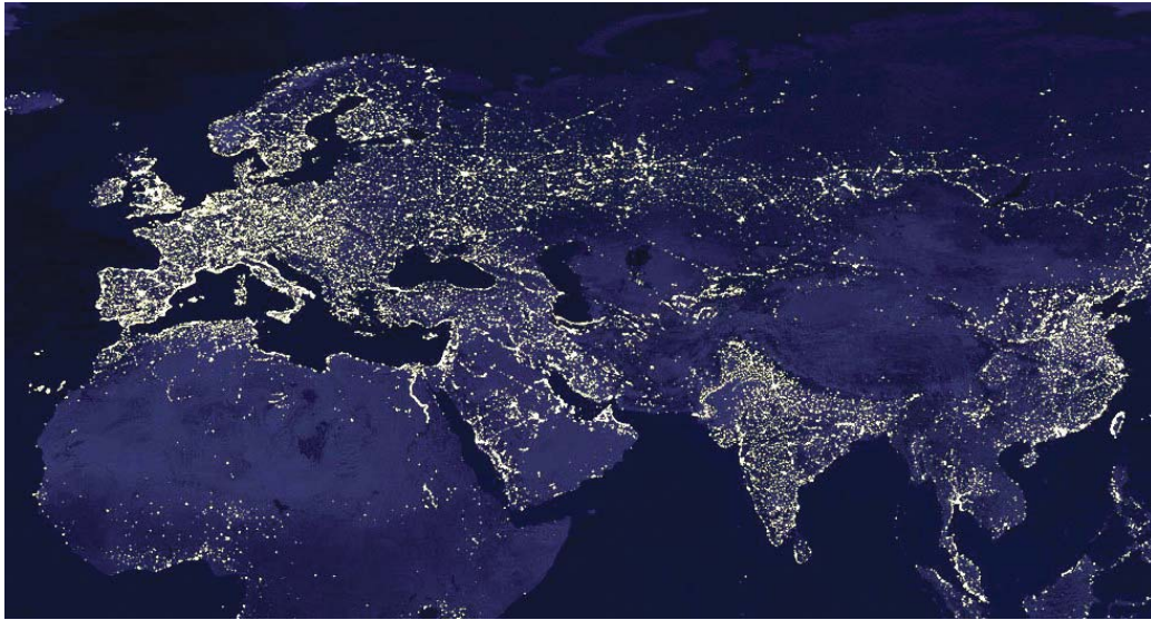
Figure 20.10 One section of a ‘night time map’ of the world produced as a composite of hundreds of images made by the Defense Meteorological Satellite Program which can detect low levels of visible/near-infrared radiance at night including lights from cities, towns, industrial sites, gas flares, and ephemeral events such as fires. Clouds have been removed. It was compiled from the October 1994–March 1995 data collected when moonlight was low (Courtesy NASA and US National Oceanic and Atmospheric Administration (NOAA))
