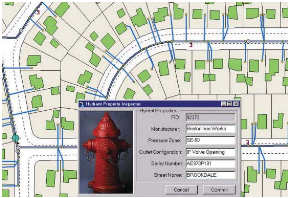
Figure 8.4 An image used as a hydrant object attribute in a water-facility system
