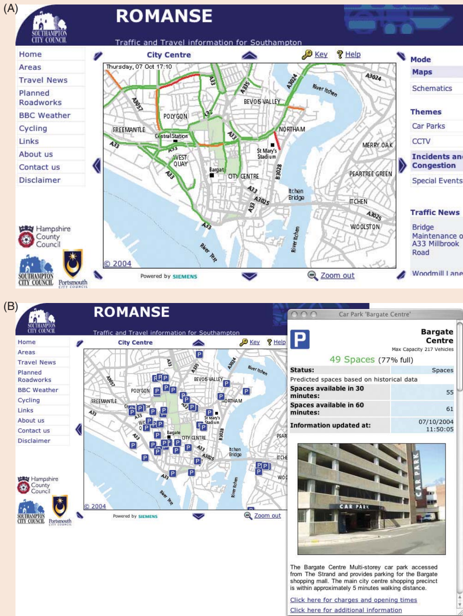
Figure 13.8 Monitoring (A) traffic flow and (B) car park occupancy in real time as part of the Web-based ROMANSE traffic management system (Base maps: Crown Copyright southampton.romanse.org.uk/ ) (Reproduced by permission of Southampton City Council)
