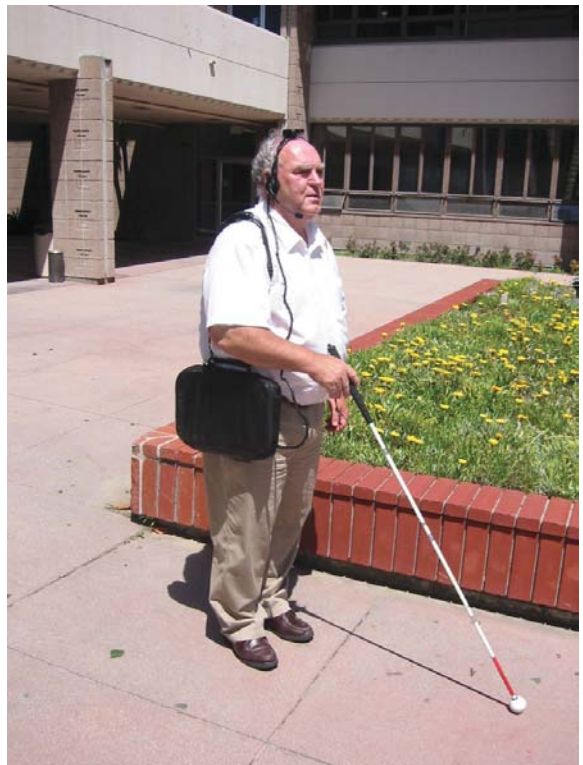
Figure 11.11 The system worn here by Reg Golledge (a leader of the development team) uses GIS and GPS to augment the senses of a visually impaired person navigating through a complex space such as a university campus (Reproduced by permission of Reg Golledge)
