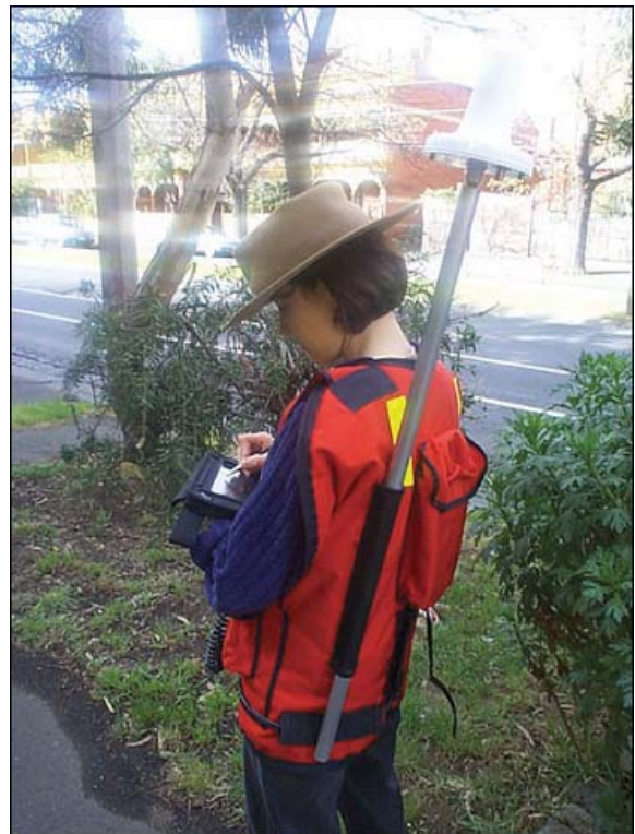
Figure 11.1 Using a simple GIS in the field to collect data. The device on the pole is a GPS antenna, used to georeference data as they are collected
