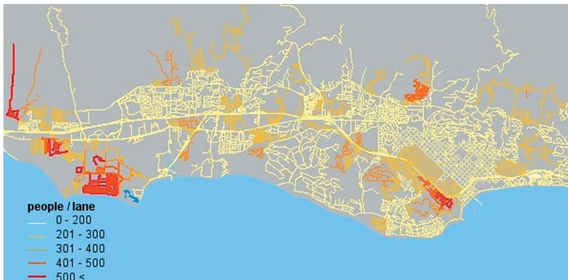
Figure 2.16 Evacuation vulnerability map of the area of Santa Barbara, California, USA. Colors denote the difficulty of evacuating an area based on the area's worst-case scenario (Reproduced by permission of Tom Cova)
