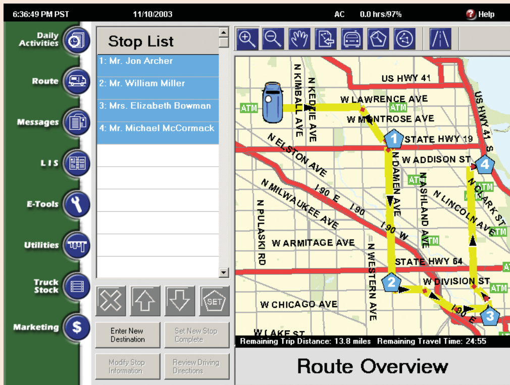
Figure 15.18 Screen shot from the in-vehicle Smart Toolbox Mapping software installed on 12,000 Sears service vehicles, showing the optimum route to the next four stops to be made by this vehicle in Chicago
