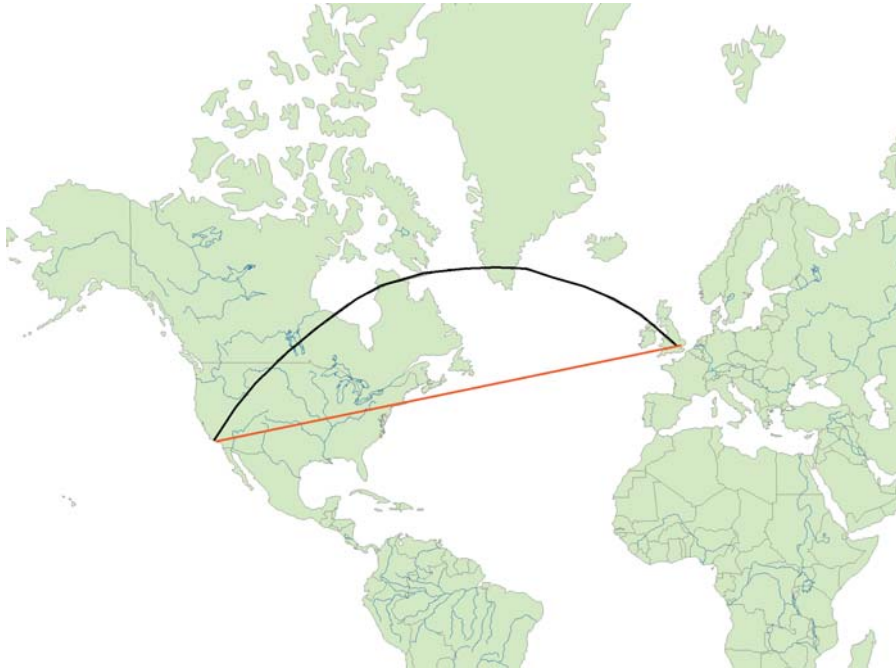
Figure 14.11 The effects of the Earth's curvature on the measurement of distance, and the choice of shortest paths. The map shows the North Atlantic on the Mercator projection. The red line shows the track made by steering a constant course of 79 degrees from Los Angeles, and is 9807 km long. The shortest path from Los Angeles to London is actually the black line, the trace of the great circle connecting them, with a length of roughly 8800 km, and this is typically the route followed by aircraft flying from London to Los Angeles. When flying in the other direction, aircraft may sometimes follow other, longer tracks, such as the red line, if by doing so they can take advantage of jetstream winds
