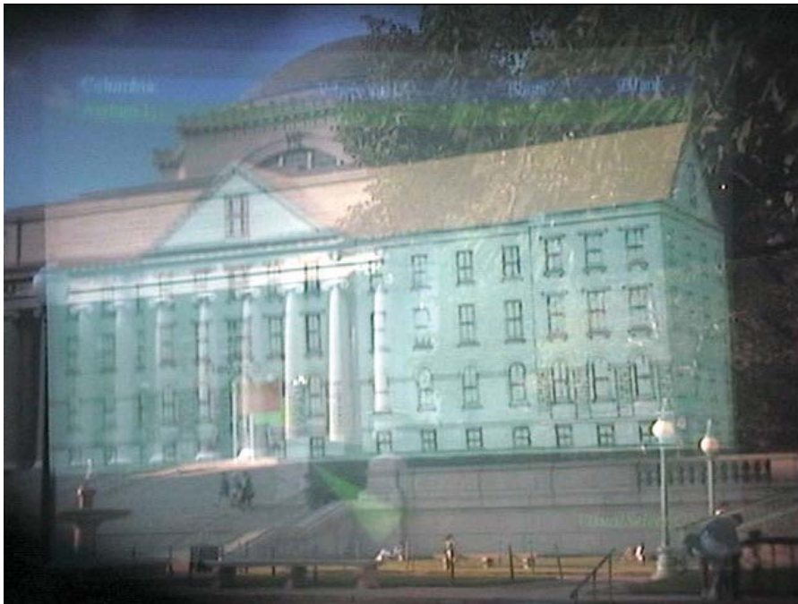
Figure 11.13 The field of view of the user of Feiner's AR system, showing the Columbia University main library and the insane asylum that occupied the site in the 1800s © 1999, T. Höllerer, S. Feiner & J. Pavlik, Computer Graphics & User Interfaces Lab., Columbia University. Reproduced with permission
