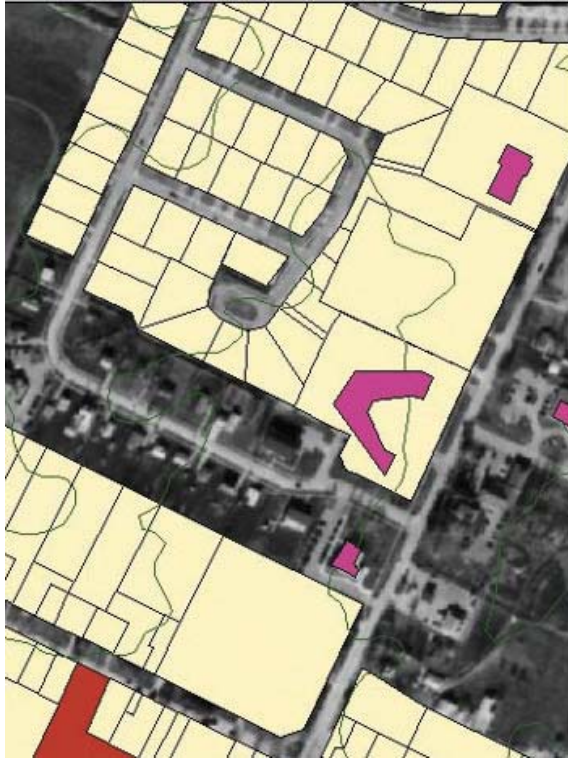
Figure 9.6 An example of raster background data (black and white aerial photography) underneath vector data (land parcels)
