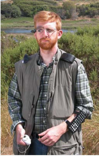
Figure 11.8 A wearable computer in use. The outfit consists of a processor and storage unit hung on the user's waist belt; an output unit clipped to the eyeglasses with a screen approximately 1 cm across and VGA resolution; an input device in the hand; and a GPS antenna on the shoulder. The batteries are in a jacket pocket (Courtesy: Keith Clarke)
