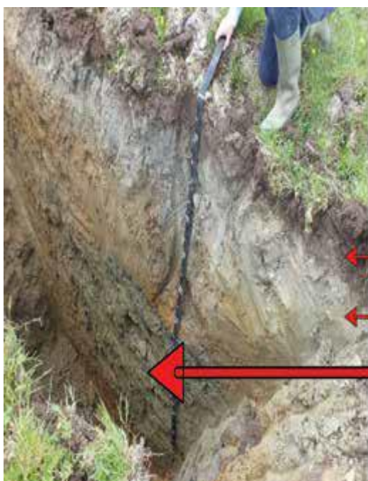
Figure 7. A typical heavy soil profile. (Left-3a) Rule of thumb: if a free draining layer is present (called “permeable layer” here) at any depth then groundwater drainage is the most appropriate solution, if not then shallow drainage (Right-3b) required
