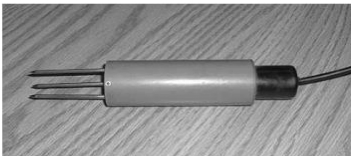
Fig. 1 A handheld capacitance type soil water content probe.
