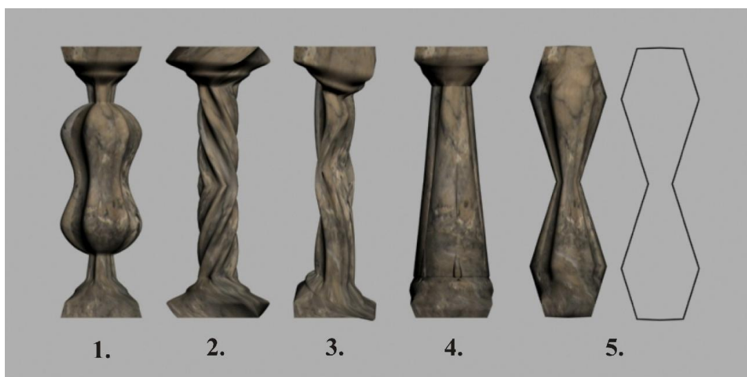
5.50-rasm. Loft obyekt deformatsiyasi: 1. Scale (Masshtab); 2) Twist (Burish); 3. Teeter (Tebranish); 4. Bevel (Qiyshaytirish); 5. Fit (Moslashtirish).
