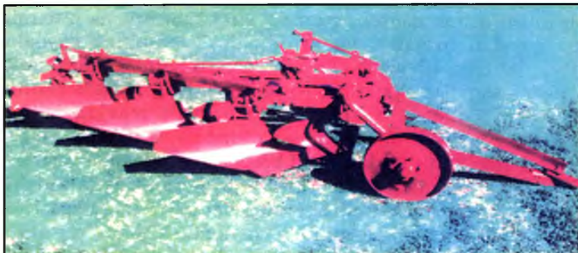
10-rasm. ПЯ-3-35 markali ikki yarusli plug
