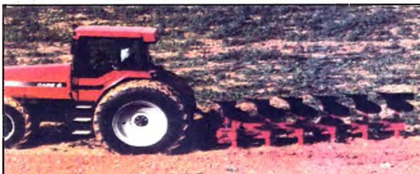
11-rasm. Six-Bottom-165 rusumli ikki yarusli universal plug
