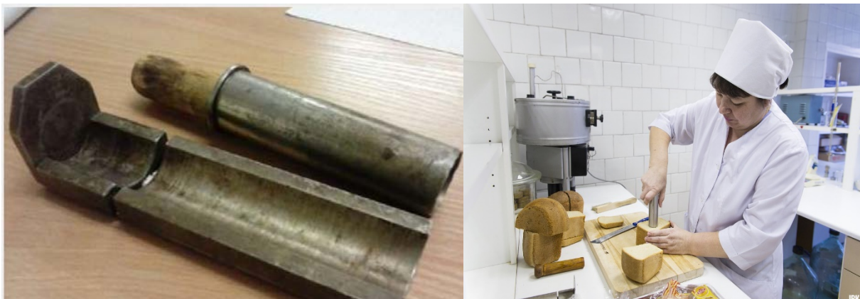
10-rasm. Nonning g‘ovakligi Juravlyova asbobi yordamida aniqlanishi.
