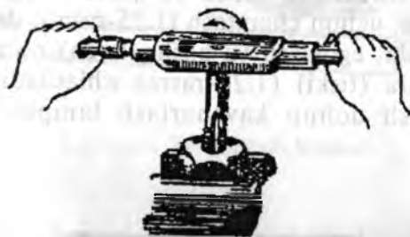
1.22-rasm. Metchik bilan rezba ochish.
