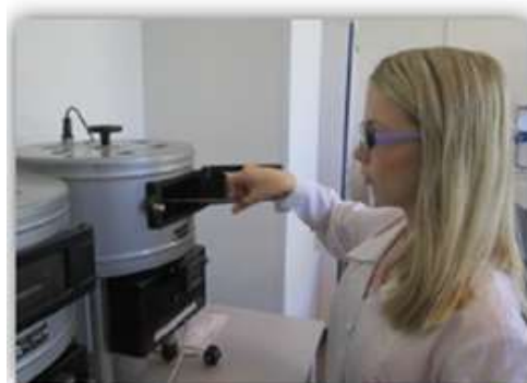
2-rasm. Quritish shkafi SESH-3Mda unning namligini aniqlash
