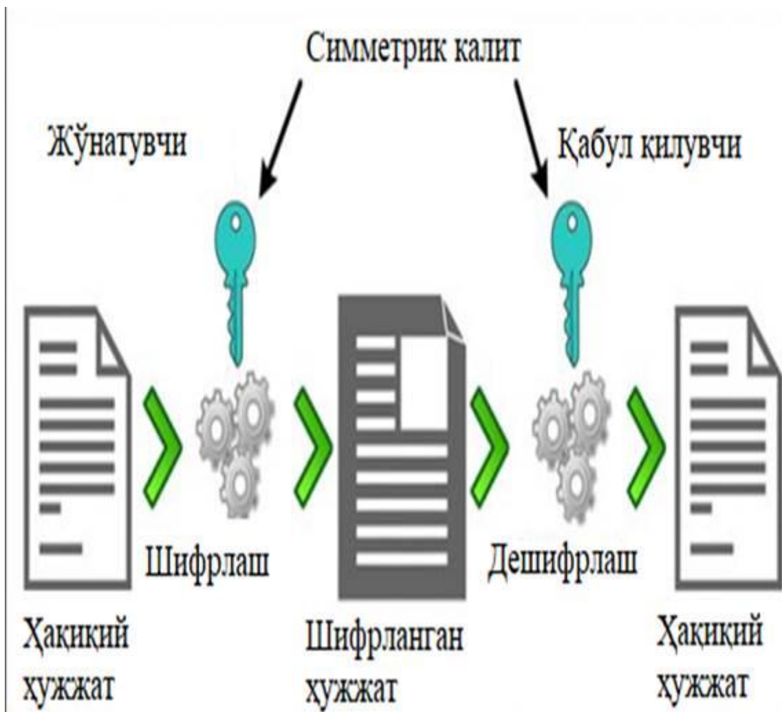
2.2-rasm. Simmetrik kalit.
