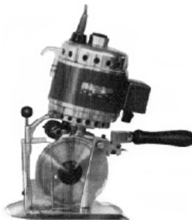
2.8-rasm. KM RS—100 disk pichoqli ko'chma bichish mashinasi.
