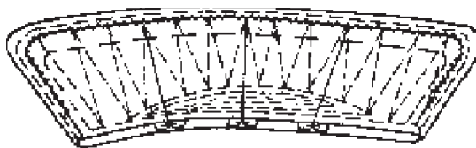
4.47-rasm. Ustki yoqani ostki yoqaga yashirin siniq baxiyali maxsus mashinada bostirib tikish.
