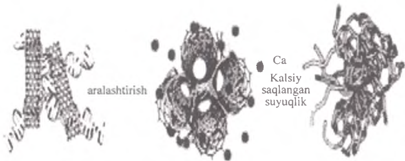
58-rasm. Uglерodli nanotrubkalar va DNK molekulasidan (rasmda chapda) tayyorlangan sun'iy nanotolani (rasmda o'ngda) olish chizmasi.
