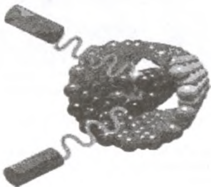
4.40-rasm. Yorug'lik ta'sirida aylanuvchi nanomotor.
