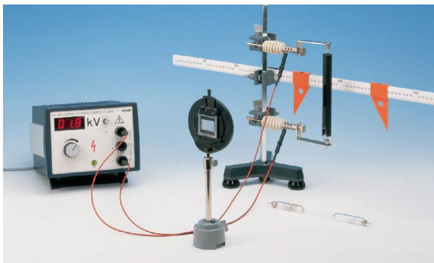
3-rasm. Vodorot atomining spektrlarini kuzatish tajriba ishi
