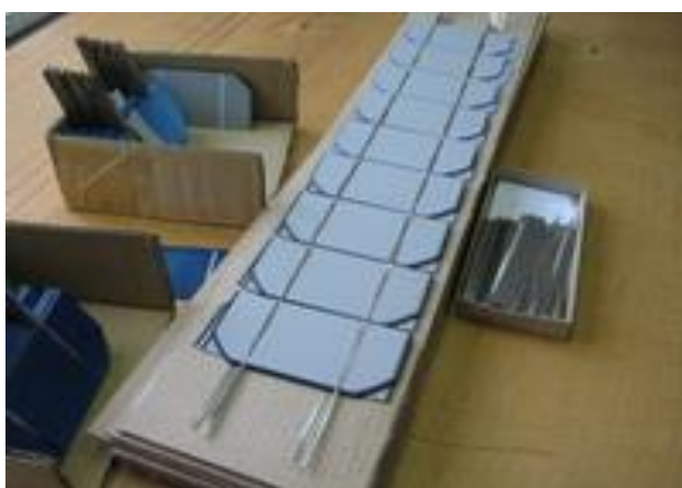
39- rasm. Modulga yig‘ish oldidan QE zanjiri
