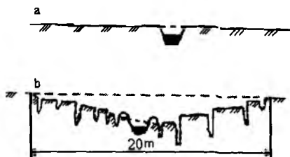
35-rasm. Sug'orish kanali qirg'og'ining cho'kish natijasida buzilishi (G'.O.Mavlonov bo'yicha). a-cho'kkanga qadar; b-cho'kkandan keyin.
