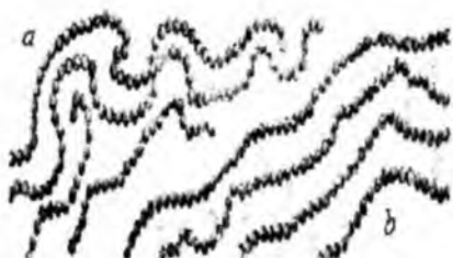
12.2-rasm. Kauchukning (a) va rezinannig (b) tuzilishi.
