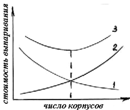
10.1 - rasm. Qurilmaning optimal sonini aniqlash.
