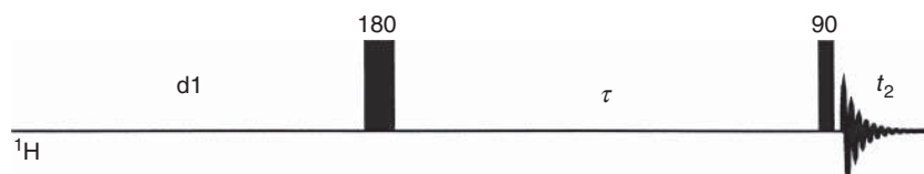
Figure 8.4 Spin-lattice ( T_1 ) inversion recovery pulse sequence. The 180^\circ pulse inverts magnetization, allowing it to recover along the z -axis. The duration of the delay, \tau , is varied from \ll T_1 to several times the longest expected T_1 relaxation time in the molecule. The resulting, varying
