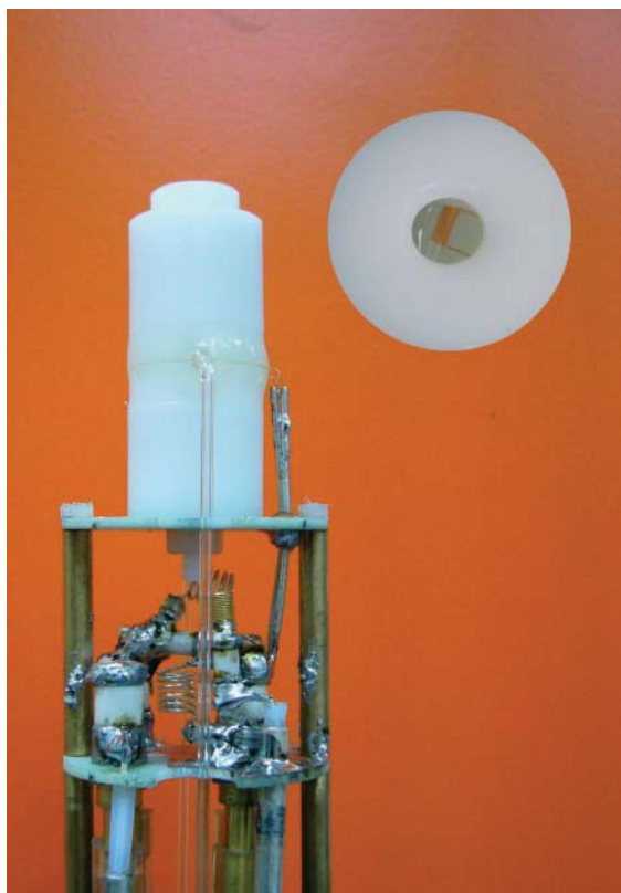
Figure 52.2 Solenoidal NMR microprobe for capillary HPLC-NMR and GC-NMR.
