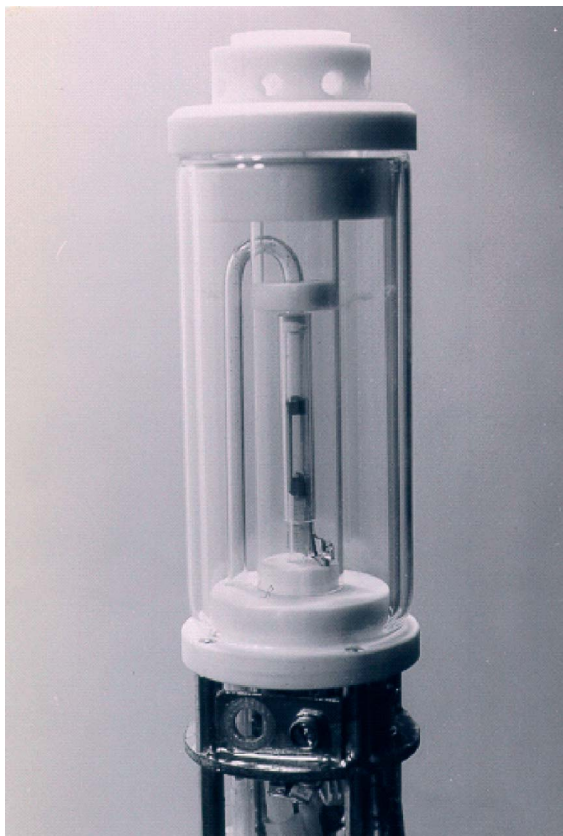
Figure 52.1 Continuous-flow ^1\text{H} NMR probe for HPLC-NMR.
