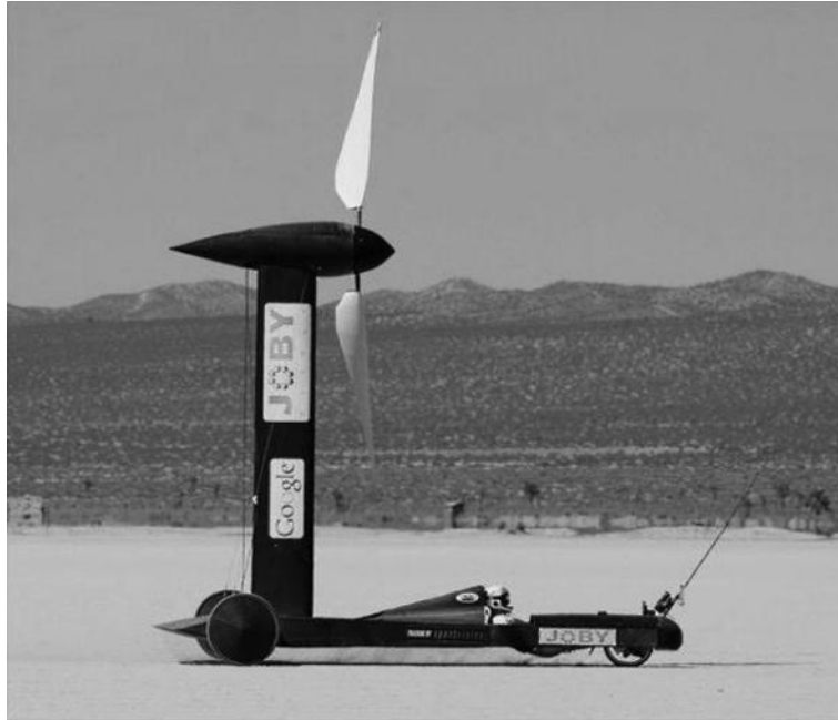
Figure 7.29 Vehicle travels directly downwind faster than the wind. (Photo of Rick Cavallaro's Blackbird; courtesy of Steve Morris.)
