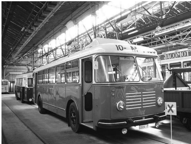
Figure 13.6 The only surviving flywheel-powered “gyrobus,” built in 1955 in a museum in Antwerp, Belgium. (Image by Vitaly Volko is licensed under the Creative Commons Attribution 2.0 Generic license, http://en.wikipedia.org/wiki/File:Gyrobus_G3-1.jpg )
