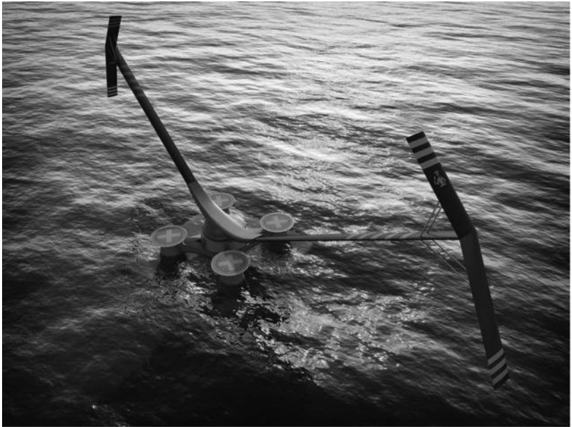
Figure 7.16 Aerogenerator X wind turbine—a proposed 10 MW design measuring 274 m tip to tip intended for offshore use. The British consortium proposing to build them, Wind power Ltd, claims that they will weigh about half as much as conventional turbines and have smaller towers and lower loads, because of the base mounting of the rotating blades. (Image provided by Windpower Ltd., Suffolk, U.K.)
