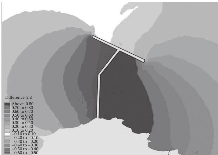
Figure 8.18 Top-down view of a dynamic tidal power T-shaped dam. The blue and dark-red colors indicate low and high tides, respectively. Note that the level of the tide is both high and low simultaneously at opposite sides of the dam. (Image is released to the public domain, http://en.wikipedia.org/wiki/Dynamic_tidal_power )
