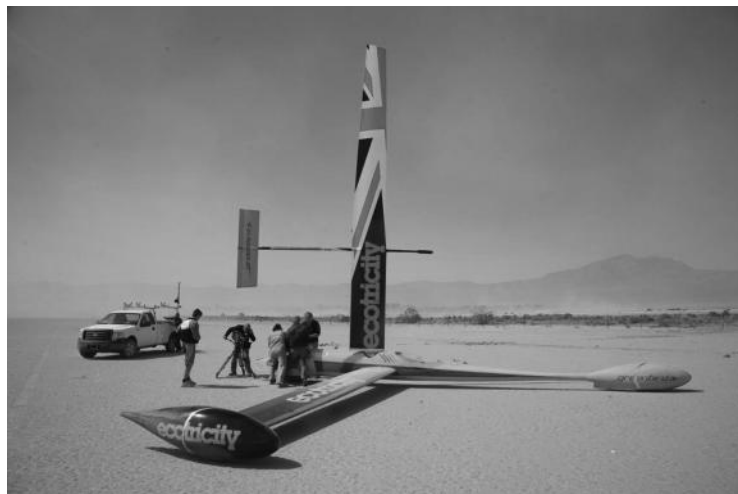
Figure 7.28 Greenbird wind-powered vehicle sets land-wind-powered speed limit in Lake Ivanpah, United States. The vertical wooden structure is a stiff sail. (Photo by Peter Lyons.)
