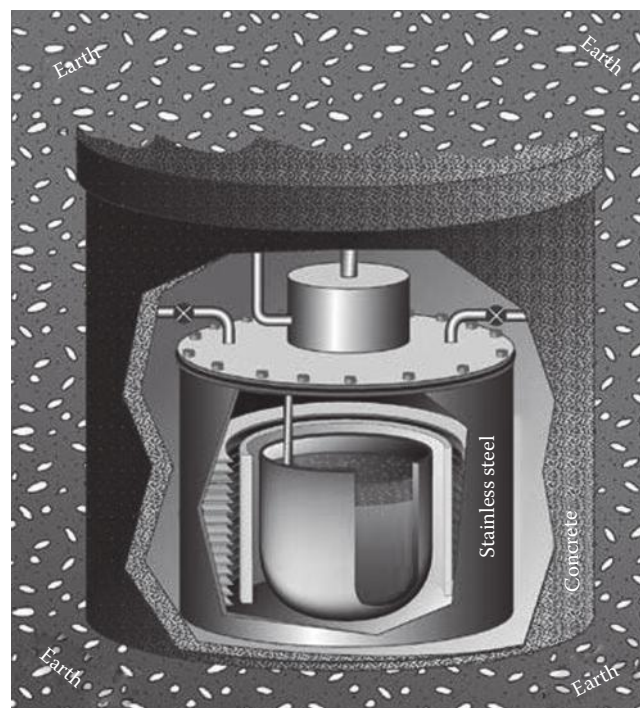
Figure 4.15 Conceptual drawing of the Hyperion “nuclear battery” (the central component of its power generating plant), which stands about the height of a man. (Courtesy of U.S. Los Alamos National Lab, a public domain image.)
