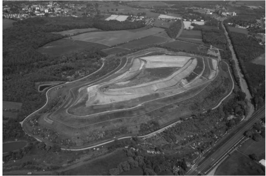
Figure 13.1 A waste heap in Hamm-Pelkum, Germany, where a power plant supplying 15–20 MW is to be installed by combining wind power with pumped storage. (Image courtesy of the German company RWE; Photo by Hans Blosssey.)
