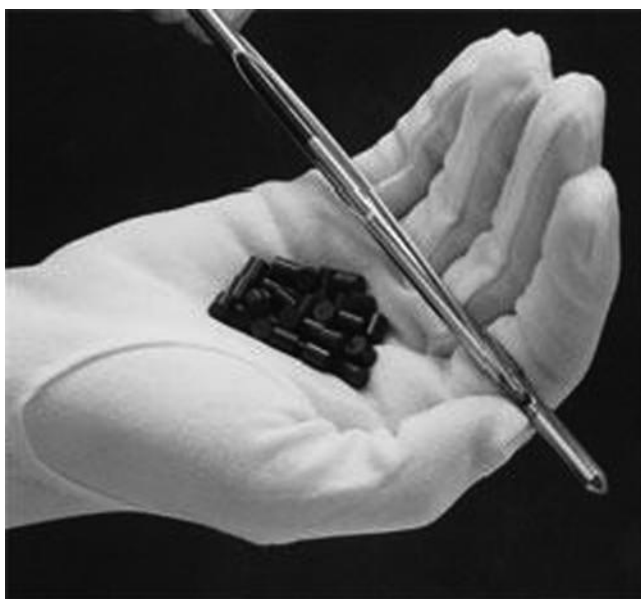
Figure 4.8 Around 20 fuel pellets for a nuclear reactor shown together with a section of a fuel rod into which they are inserted. One of those tiny pellets contains the energy equivalent of nearly a ton of coal. (Image courtesy of the U.S. Department of Energy, Washington, DC, is in the public domain.)
