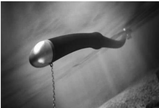
Figure 8.13 As a wave passes the Anaconda made by Checkmate Sea Energy, it creates a pressure pulse (see the bulge) that travels down the length of it. (Image courtesy of Francis J.M. Farley.)
