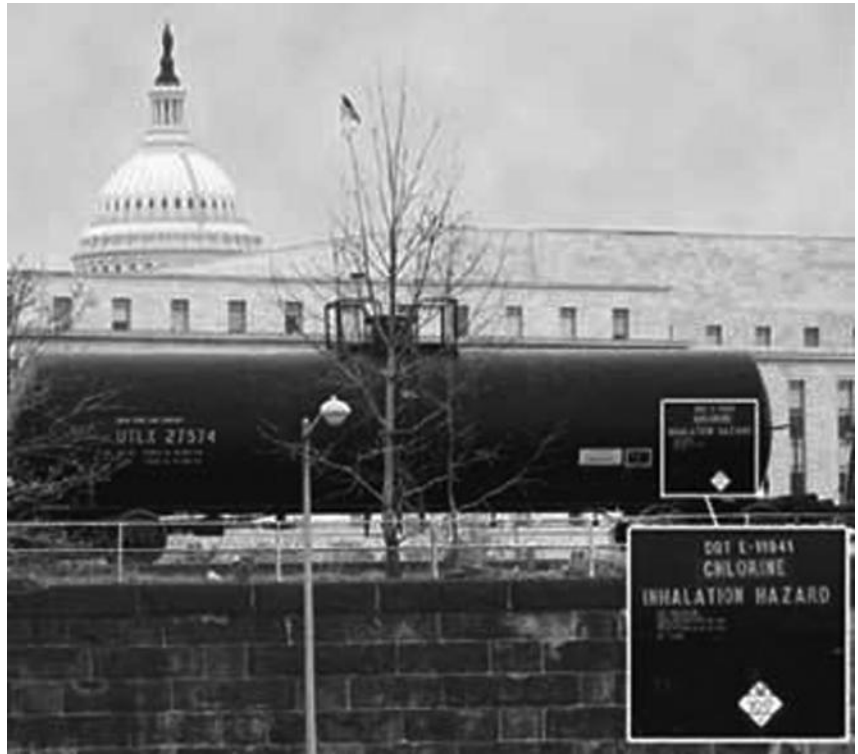
Figure 4.13 Shipment of a 90 ton pressurized chlorine gas rail tank within four blocks of the Capitol building in Washington, DC. Helpfully (to terrorists), the nature of the cargo is clearly labeled with a sign on the side, and there are no obvious armed guards onboard. (Photo courtesy of Jim Dougherty, Sierra Club, 2004.)
