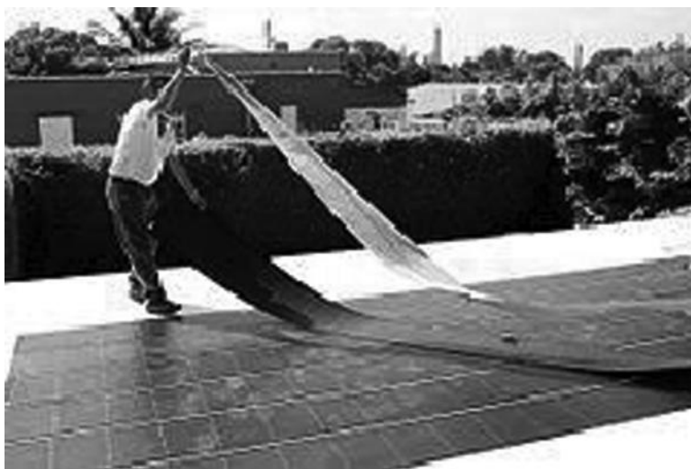
Figure 11.19 Flexible sheets of thin-film solar cells. (Image created by Fieldsken Ken Fields is licensed under the Creative Commons Attribution-Share Alike 3.0 Unported license, http://en.wikipedia.org/wiki/Thin_film_solar_cell )
