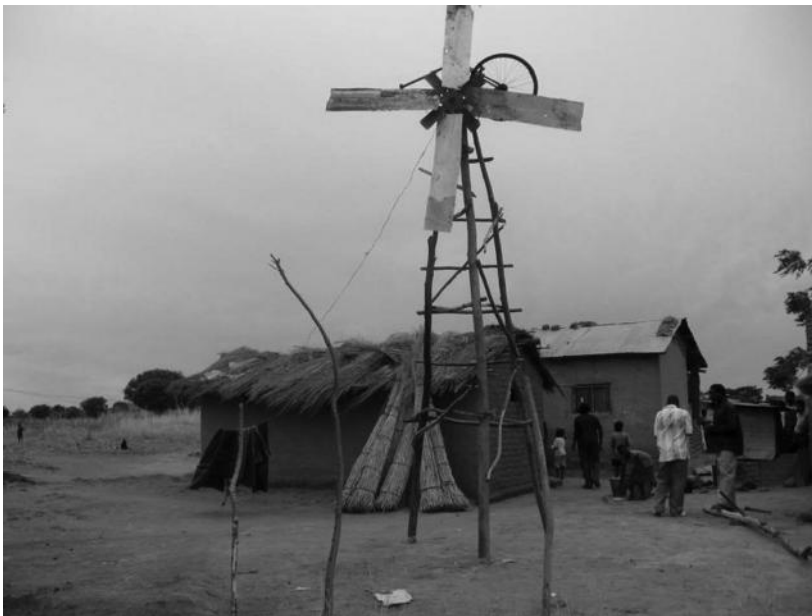
Figure 7.18 Makeshift wind turbine assembled using bicycle parts and materials collected in a local scrap yard by a boy in Malawi. (Image by Erik (HASH) Hersman is licensed under the Creative Commons Attribution 2.0 Generic license, http://en.wikipedia.org/wiki/William_Kamkwamba )
