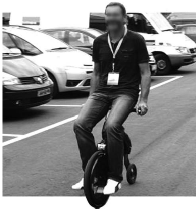
Figure 12.2 The YikeBike—a highly unusual type of folding electric motor bike capable of speeds up to 25 km/h—is the smallest and lightest such vehicle in the world, weighing only 22 lb and small enough to fit in a backpack. Unfortunately, it is not believed to be street-legal anywhere in the world, and also comes at a fairly steep price ($3000). (Image created by Anna Frodesiak is in the public domain, http://en.wikipedia.org/wiki/YikeBike )
