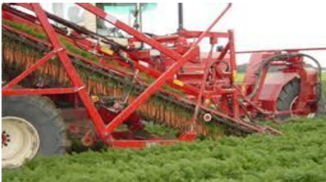
1.51-rasm. Sabzi yig‘ish Ye-825 kombaynning ish jarayonidagi ko‘rinishi.
