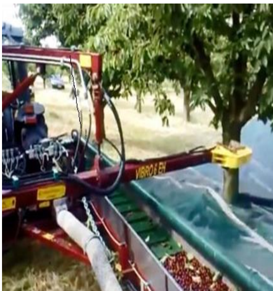
1.33-rasm. Danakli mevalarni yig'ib olishda qo'llanadigan Germaniyaning VIBROEH rusumli agregatining ish jarayoni
