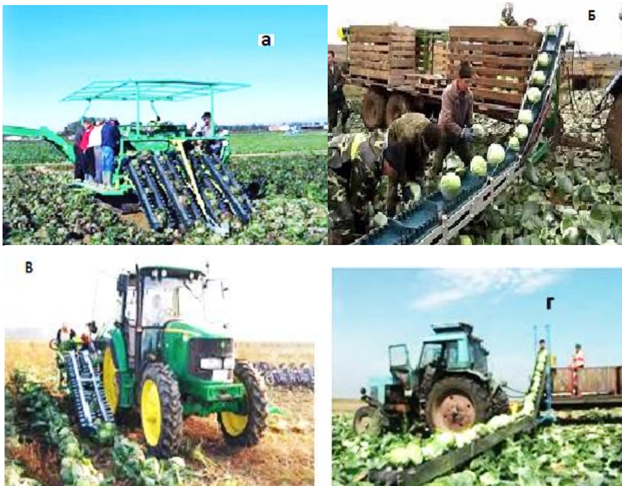
1.49-rasm. Karam yig‘ish (A, V) va uni sirtqi barglaridan tozalab transport vositasiga yuklash (B, G) jarayonlari.
