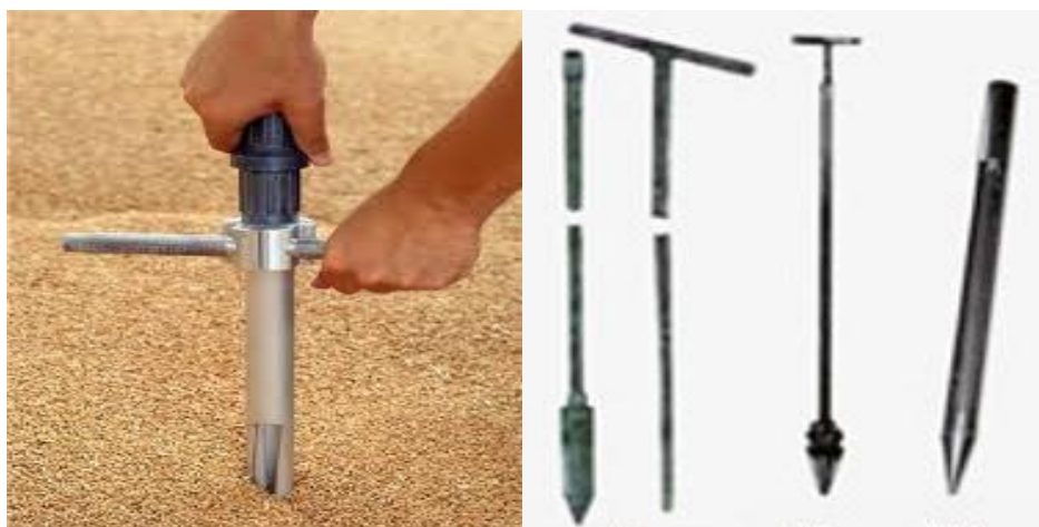
1-rasm. Don shuplari va cho`mich. 1-vagon konus shuplari; 2-qop shupi; 3- silindr shup; 4-cho`mich
