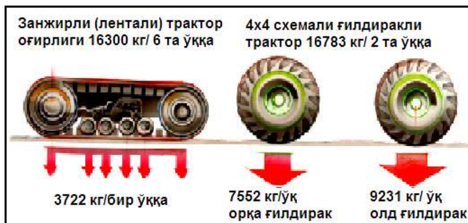
1.18-rasm. Traktor yurish qismining tuproqning chuqurzichlanishiga ta'siri
