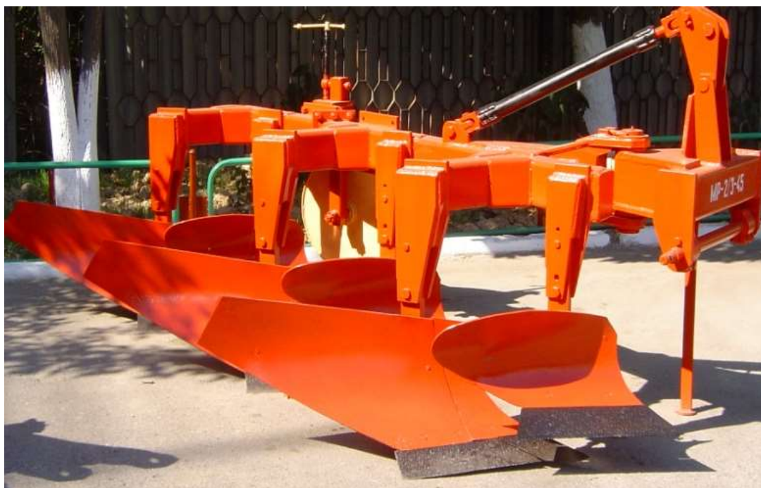
2.3-rasm. Ikki yarusli plug
