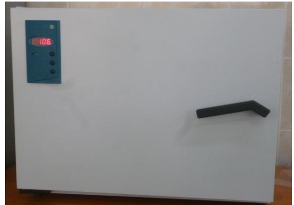
15-rasm. Olingan tuproq na'munalarini termostatda (quritish shkafi) quritish.
