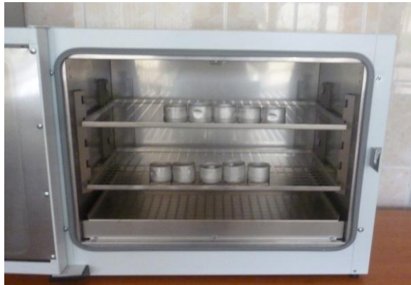
15-rasm. Olingan tuproq na'munalarini termostatda (quritish shkafi) quritish.
